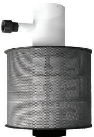
Perforated Stainless Screen .117" Perf. 16ga 316SS
